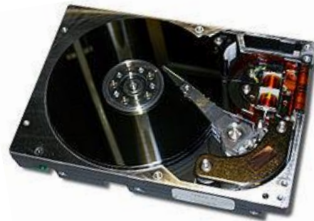
Disk drive with GMR head 2000's
