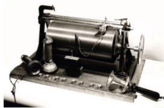
Magnetic wire recorder 1880's
