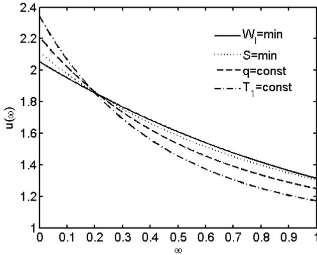
FIG. 7: Dependence of the ratio of the reservoir temperature to the system temperature  $u(\omega)$  on the dimensionless time  $\omega$  in case of the heat transfer law  $q \propto (\Delta(T^4))^{1.25}$
