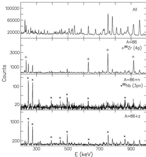
FIG. 8: Comparison of the effectiveness of using ion chamber and neutron detectors to separate the  $3pn$  channel from the  $4p$  channel in the  $A = 86$  gated data.
