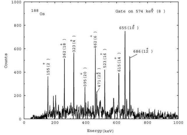
FIG. 9: Gamma ray coincidence spectrum for  $^{188}\text{Os}$  nucleus gated on 574 keV transition.
