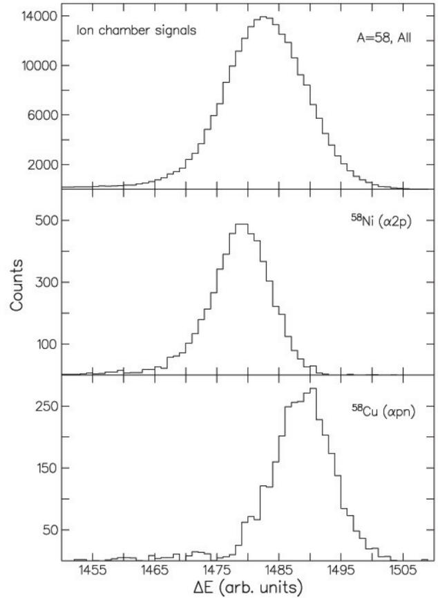
FIG. 6: Ion chamber signals of the isobars.
