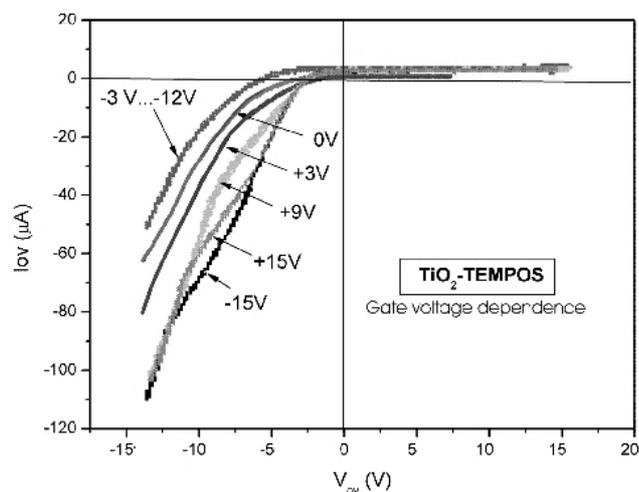
FIG. 4: Current/voltage characteristics of a  $\text{TiO}_2$ -TEMPOS structure. In this peculiar case, the gate voltage influences only the third quadrant. Interestingly, both high positive and negative gating voltages change the current/voltage characteristic in the same way, but lower gating voltages do not. Photocatalytic effects (not shown here) change only the curve in the first quadrant and remain nearly unaffected by the gating signals.
