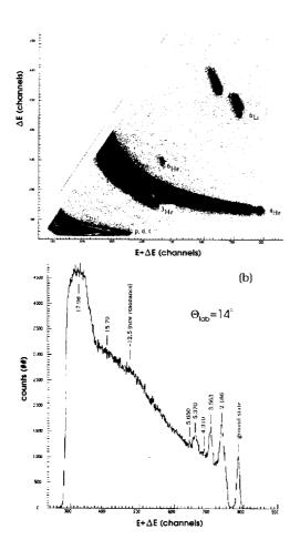
Figure 1. (a)Typical particle identification  $E - \Delta E$  spectrum for the  ${}^{3}He({}^{7}Li, \alpha){}^{6}Li$ . (b)Projection of the  $\alpha$ -particles events onto the total energy axis ( $E + \Delta E$ ). The excitation energies of  ${}^{6}Li$  are indicated in MeV.
