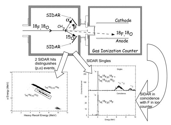
Figure 1. A mixed  $^{18}$ F/ $^{18}$ O beam bombarded a polypropylene target. Recoil  $\alpha$  and  $^{15}$ O ions were detected in coincidence in SIDAR, while beam-like  $^{18}$ F recoils were detected in an ionization counter and in coincidence with scattered protons.
