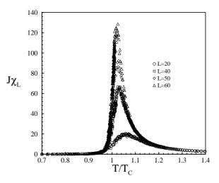
Figure 6. Plots of the dimensionless magnetic susceptibility  $(J\chi_L)$ , versus the scaled temperature (same scale as in Fig. 5), for the ferromagnetic Ising model on square lattices of different linear sizes.
