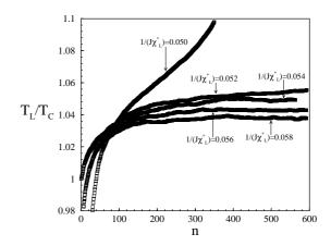
Figure 1. Evolution of the temperature [in units of the corresponding exact critical temperature (see Table 1)] with the iteration step n, for different choices of  $\chi_L^*$ , for the ferromagnetic Ising model on a square lattice of linear dimension L = 20. Among the choices investigated, the optimal choice corresponds to  $1/(J\chi_L^*) = 0.054$ , leading to the stationary temperature  $T_L^*/T_c = 1.0488 \pm 0.0022$ .
