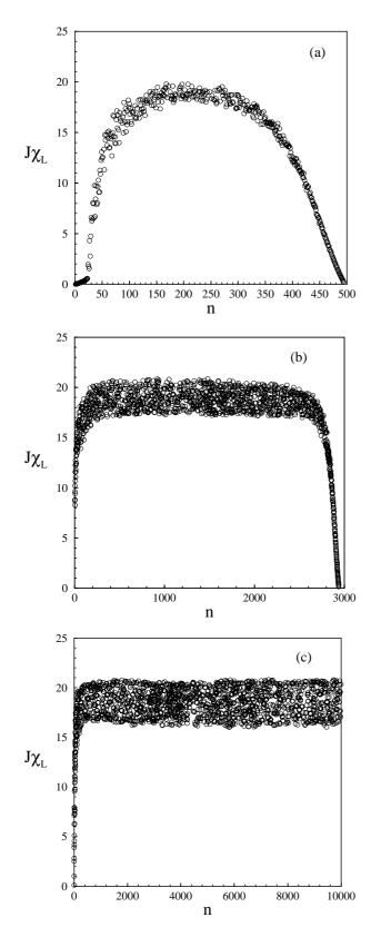
Figure 2. Evolution of the dimensionless magnetic susceptibility with the iteration step n, for some of the choices of  $\chi_L^*$  of Fig. 1, for the ferromagnetic Ising model on a square lattice of linear dimension L = 20. (a)  $1/(J\chi_L^*) = 0.050$ ; (b)  $1/(J\chi_L^*) = 0.052$ ; (c)  $1/(J\chi_L^*) = 0.054$ . Among the choices investigated, the optimal choice corresponds to  $1/(J\chi_L^*) = 0.054$ .
