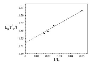
Figure 4. Extrapolation of the finite-size stationary temperatures  $T_L^*$ , calculated through the recursive-search method, to the  $L \to \infty$  limit, for the ferromagnetic Ising model on a honeycomb lattice. The extrapolated stationary temperature is  $k_B T^*/J = 1.518 \pm 0.006$ .
