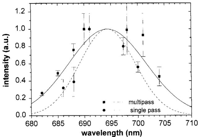
Figure 3: Thomson scattering profiles. Experimental results are represented by points and best theoretical fitting by curves. The measurements were performed for different times  $t$  after beginning of the discharge. For single pass ( $t = 3 \mu\text{s}$ ):  $n_e = (1.3 \pm 0.2) \times 10^{22} \text{ m}^{-3}$ ,  $T_e = (15 \pm 4) \text{ eV}$ ; for multipass ( $t = 5 \mu\text{s}$ ):  $n_e = (5.7 \pm 0.5) \times 10^{21} \text{ m}^{-3}$ ,  $T_e = (26 \pm 4) \text{ eV}$ .
