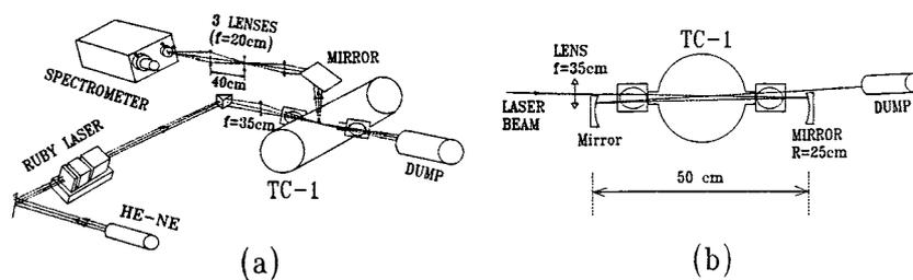
Figure 1: a) Thomson scattering system on TC-1. b) Details of the multipass system.
