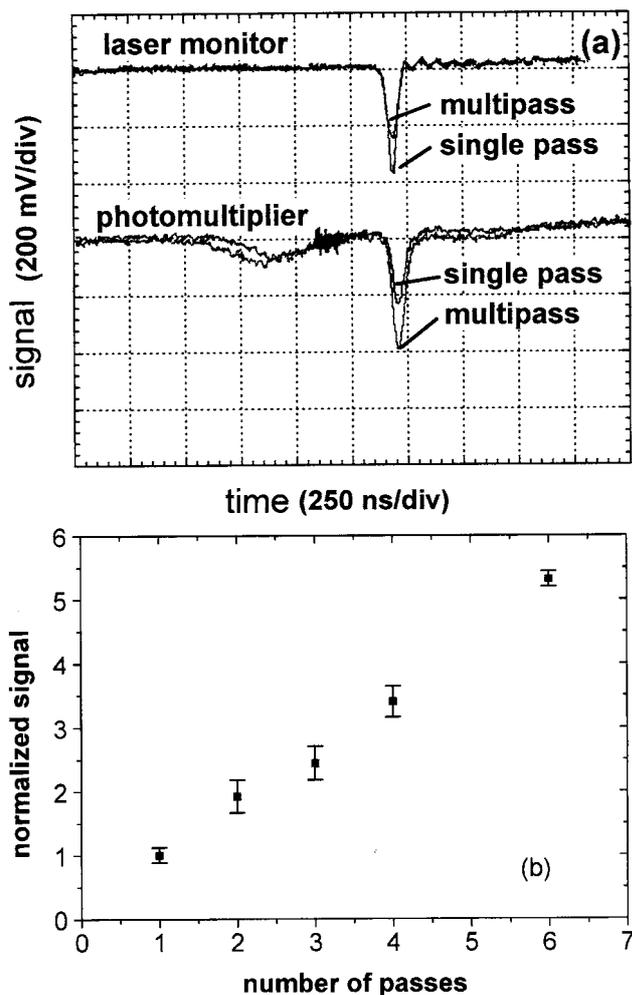
Figure 2: a) Comparison between single pass and multipass Thomson scattering. The upper signal is the laser monitor and the lower signal is the plasma continuum and Thomson signal ( $\lambda = 688.0$  nm). b) Normalized signal as function of the number of passes.
