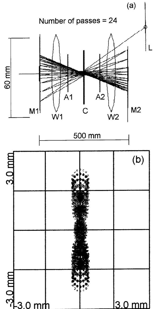
Figure 4: a) Multipass system for the tokamak NOVA. L is the focusing lens,  $M_1$  and  $M_2$  are the reflecting mirrors,  $W_1$  and  $W_2$  the entrance windows,  $A_1$  and  $A_2$  the aperture limitation of the chamber and  $C$  is the center plane of the scattering region. b) Cross section of the laser beam in the center plane  $C$ .
