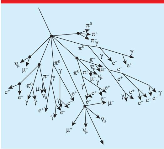
**Figure 3.** Schematic view of an atmospheric air shower. The particles shown are examples that are not in real proportion to the particles produced in a shower. The lateral size of a shower at the level of the Pierre Auger Observatory depends strongly on its arrival direction, energy and particle type. Therefore, this schematic view might not be in scale for some specific showers.
