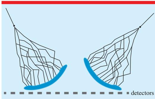
**Figure 6.** Shower development. Two showers are shown, each shower coming from a different direction. The figure illustrates how different shower directions generate different hit time patterns on the surface detectors.
