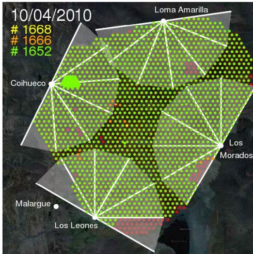
**Figure 1.** Pierre Auger Observatory. The white lines represent the field of view of the fluorescence telescopes. The map shows the status of the observatory on 10 April 2010. The dots of different colours represent the surface detectors. Each colour represents an operational status of the detectors.
