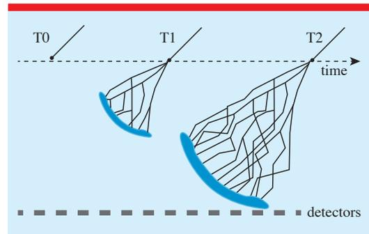
**Figure 5.** Shower development. The figure shows one air shower in three different development stages. The black boxes represent the detectors of the Pierre Auger Observatory. The blue area represents the spread of the particles in the shower front. Not to scale.
