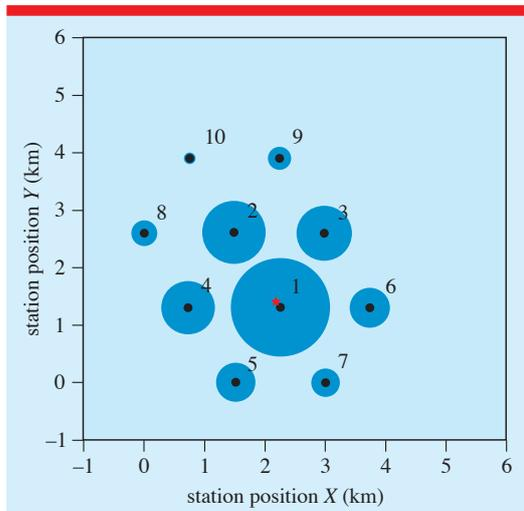
**Figure 4.** Schematic representation of the positions of the stations hit by a shower and their corresponding signals (see text). The detectors are numbered according to table 1.
