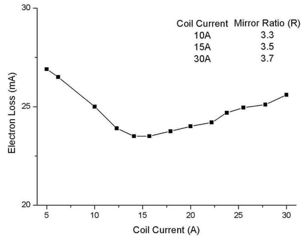
Figure 5. Electron axial flow collected by positive bias end disk as a function of mirror ratio.
