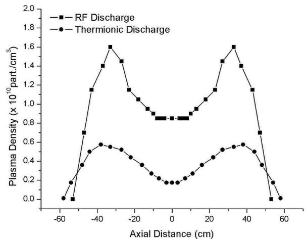
Figure 6a. Axial plasma density profile for RF discharge compared with thermionic discharge.
