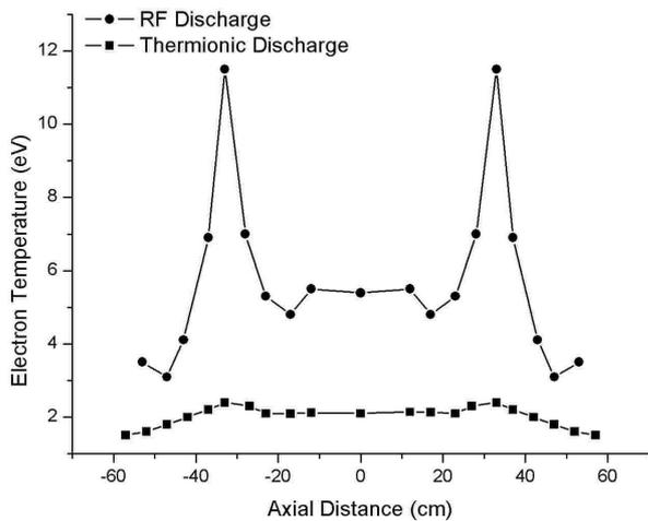
Figure 6b. Axial electron temperature profile for RF discharge compared with thermionic discharge.
