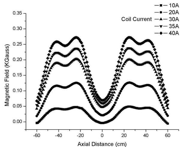
Figure 2a. Axial space profile of magnetic field measured by Hall probes.
