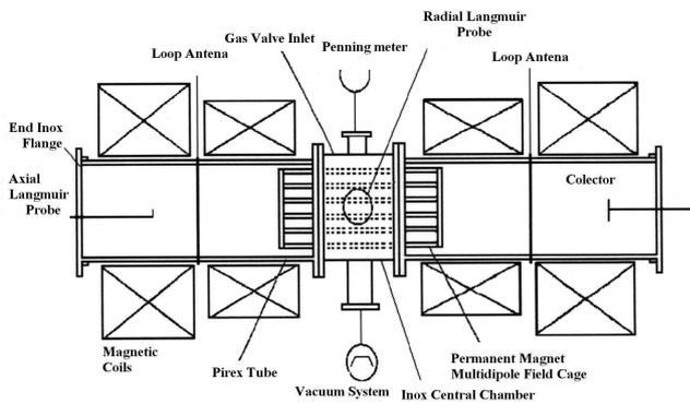
Figure 1a. Magnetic mirror machine, general schematic.
