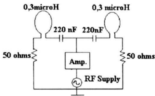
Figure 3a. Schematics of RF circuit with loop antennas.
