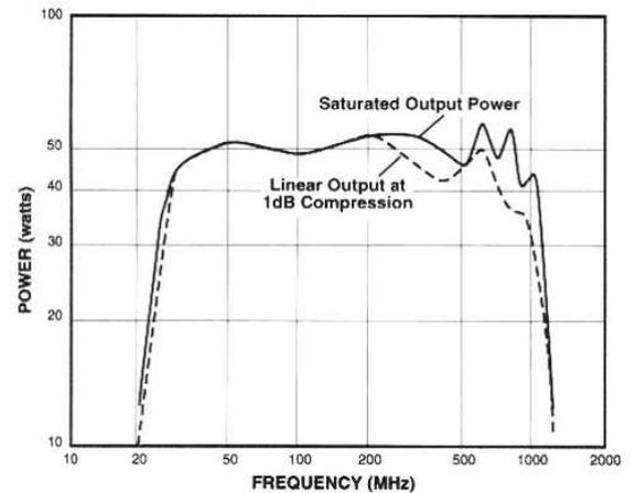
Figure 3b. RF amplifier power curve.
