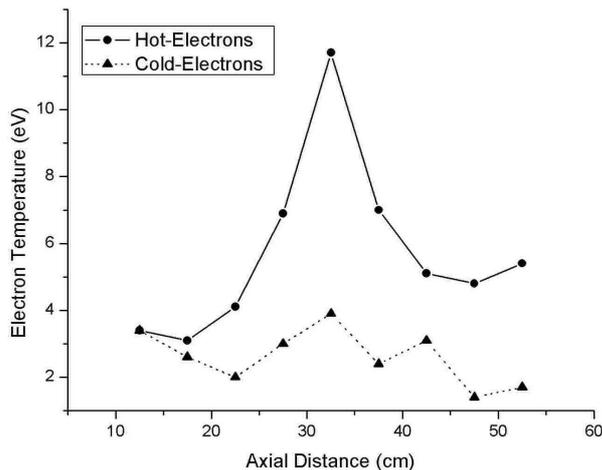
Figure 7. Two electron temperature plasma at the mirror throat.
