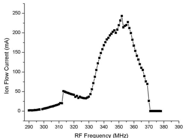
Figure 8b. Ion axial flow collected by a disk negatively bias probe versus RF frequency.
