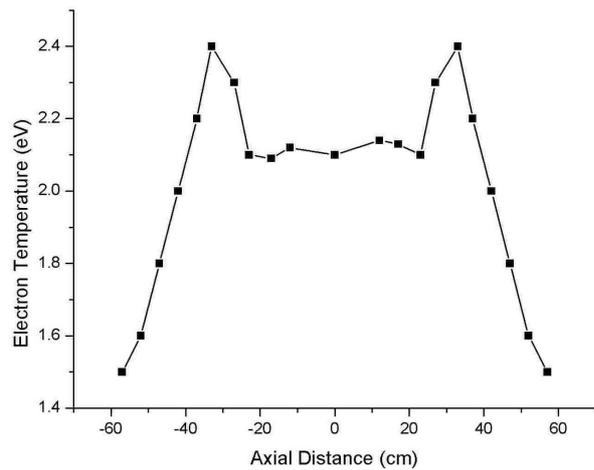
Figure 4b. Axial electron temperature profile: Thermionic discharge.
