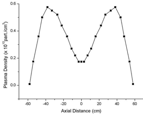
Figure 4a. Axial plasma electron density profile: Thermionic discharge.
