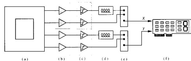
Figure 7. X-ray detection system block diagram including detector (a), pre-amplifiers (b), discriminators (c), delay generators (d), time-to-amplitude converters (e) and the image acquisition interface (f).
