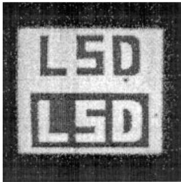
Figure 9. Image obtained by illumination of the detector with an  $^{55}\text{Fe}$  x-ray source, through a lead tape mask containing the letters L, S, and D.]
