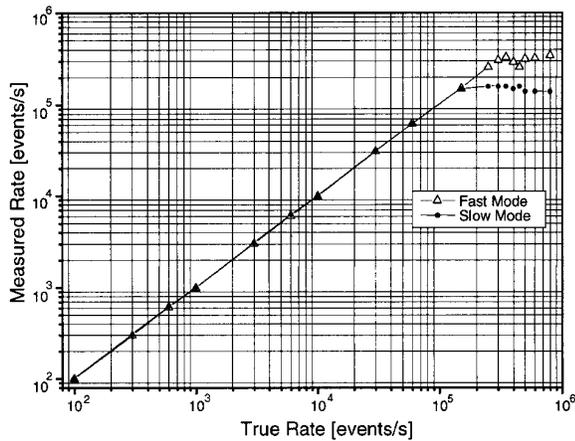
Figure 5. Acquisition rate measurement results.
