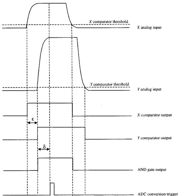
Figure 1. Timing signals diagram.
