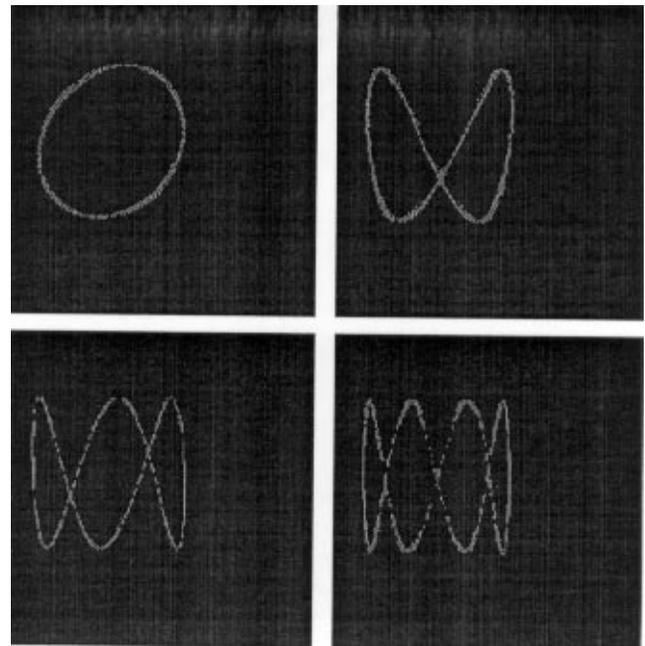
Figure 6. Examples of Lissajous patterns scanned by the image acquisition interface. Sine waves frequencies are multiples of 1 KHz, while the sampling rate frequency provided by the external trigger is 360 KHz.
