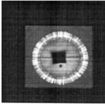
Figure 8. Laue diffraction pattern for a polycrystalline powder sample. Dark region in the center is the beam stopper mask shadow.
