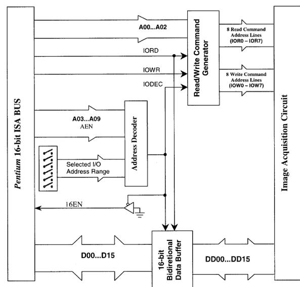
Figure 3. Details of the communication between the PC bus and the interface circuit.
