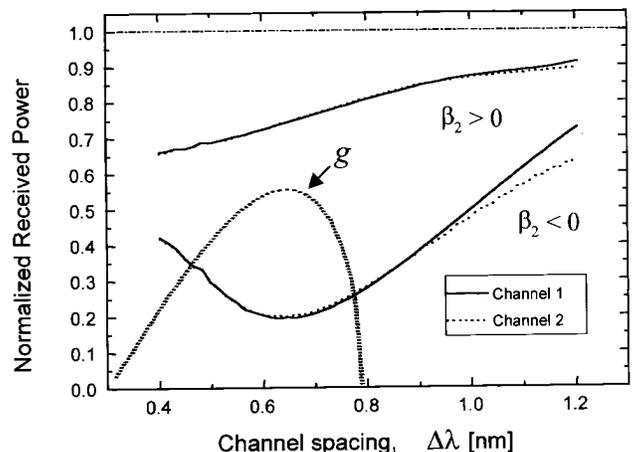
Figure 1. Normalized Received Power as a function of channel spacing (MI gain spectrum  $g$  is also shown for comparison).
