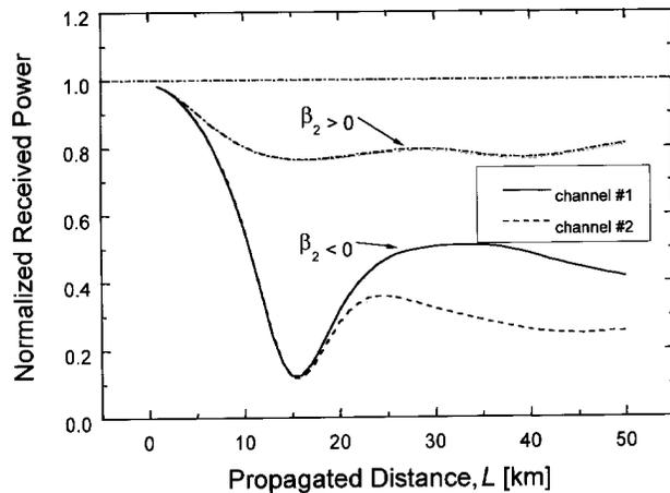
Figure 2: Normalized Received Power as a function of propagated distance.
