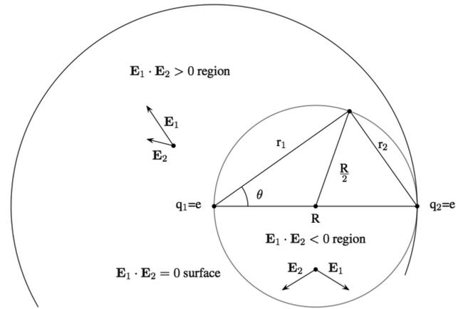
Figure 2 - The distribution of the electrostatic energy density for two similar positive point charges.
