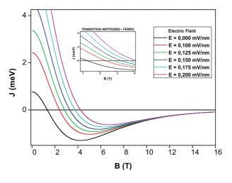
FIG. 1: Exchange energy J(B) in *meV* plotted against the magnetic field for different electric fields, for  $a = 0.7a_b$  and c = 2.36. The most remarkable feature of J is the change of its sign from positive to negative.
