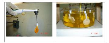
FIG. 4: Details of the oscillating device (tooth-brush), the sampleholder and the chemical bath. Clean CdS films and transparent chemical bath was obtained after deposition with this device.
