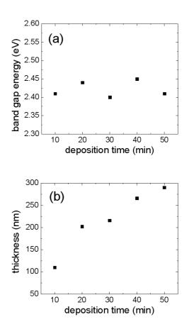
FIG. 2: Properties of the CdS films deposited with substrate oscillation + magnetic agitation: (a) band gap energy and (b) film thickness obtained as a function of deposition time.
