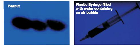
FIG. 11: Thermal neutron radiographic images cast on the converter-scintillating screen and caught by a conventional 50 mm / f 1.8 photographic camera using an ASA 400 film and an exposition time of 30 seconds.
