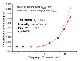
FIG. 2: Effect of variable wing length  $t_1$  on the probability for 2photon absorption in Helium, same field conditions as in figure 1, except that, while t<sub>2</sub> (the duration of the flat part of the pulse) is kept constant at 100 atomic units, the FWHM given by  $t_1+t_2$  is, of course, not the same for each point. The squares show the effect of rectangular pulses with time duration  $t_1+t_2$ .
