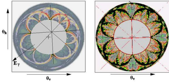
Figure 2. (Left) Simulated scan illustrating the alignment procedure by fitting a template. Here the face of the crystal, i.e. the [100] plane, is offset in  $\theta_v$  and  $\theta_h$  with respect to the direction of the incident electron beam. (Right) Final scan taken during a data scan run. We see that the crystal is aligned to the desired degree of precision.
