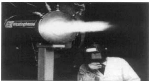
Figure 8. Photograph of a high power plasma torch, manufactured by Westinghouse [10].
