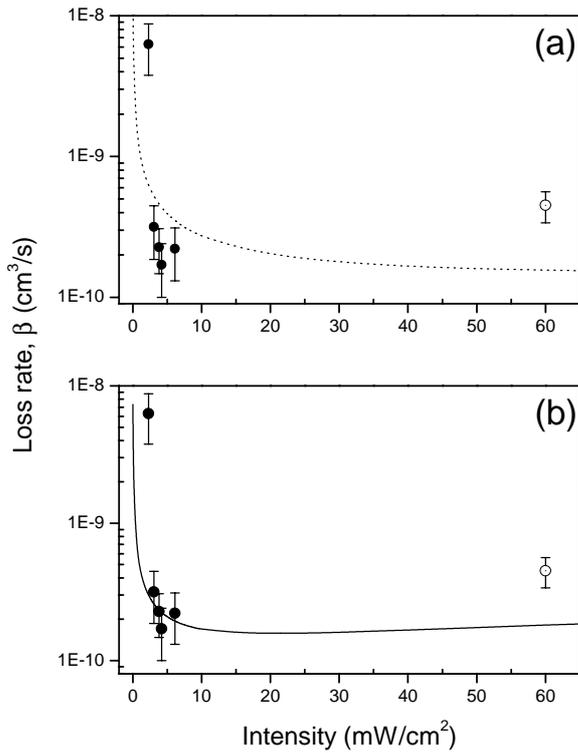
Figure 5. Plot of the loss rate coefficient as a function of the trap laser light intensity. (a) Comparison of the experimental and model results for the case where the linewidth,  $\Gamma_M$ , is constant with the internuclear separation. (b) Comparison with the improved model for the case where the linewidth depends on the internuclear separation.
