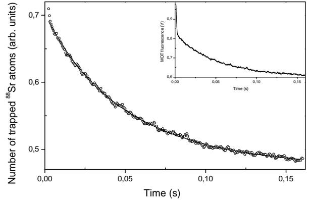
Figure 3. Comparison between the fitting generated by the eq.6 and the smoothed unloading curve. In the inset plot, we show a typical full unloading curve, this curve was obtained by a sudden change of the MOT laser intensity.
