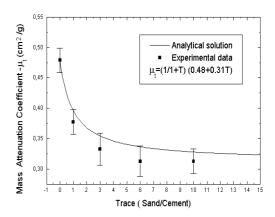
Figure 4. Solid line shows the theoretical dependency between the trace used in the concrete samples with the mass attenuation coefficients of gamma ray ( $cm^2/g$ ). The experimental points were obtained by tomographic techniques using the samples with the proportion between sand and cement, described in the text.
