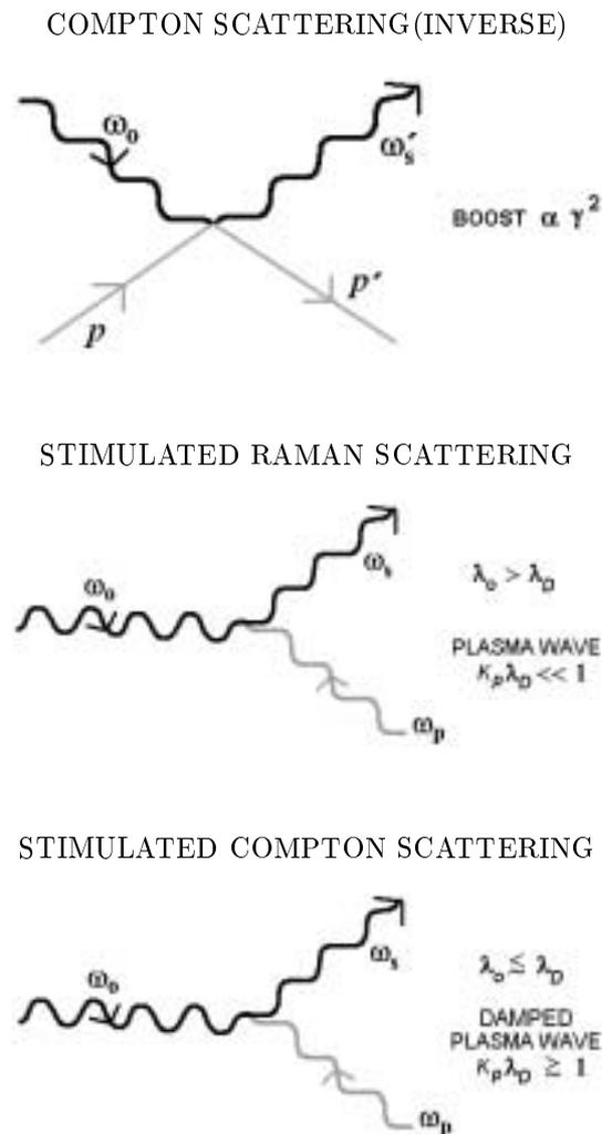
Figure 2. Scattering of radiation in a plasma.
