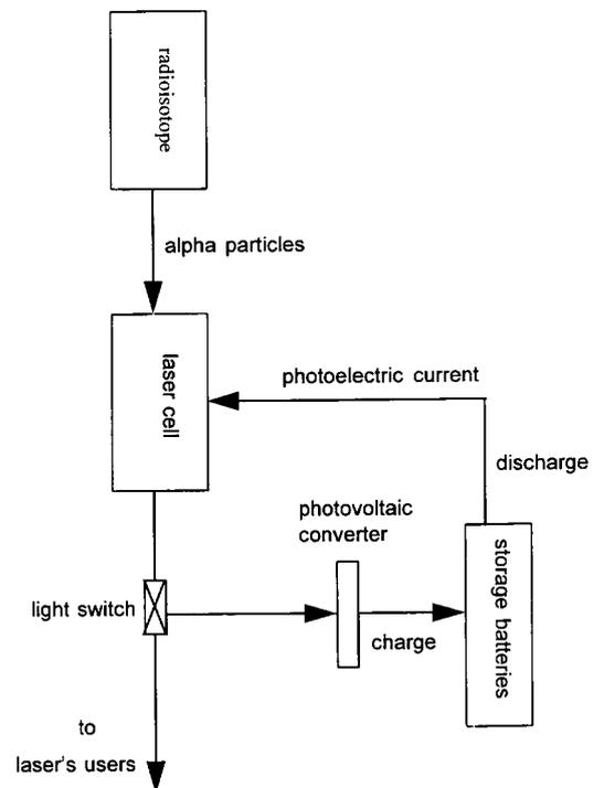
Figure 1. A proposed energy feed back for radioisotope laser generator.
