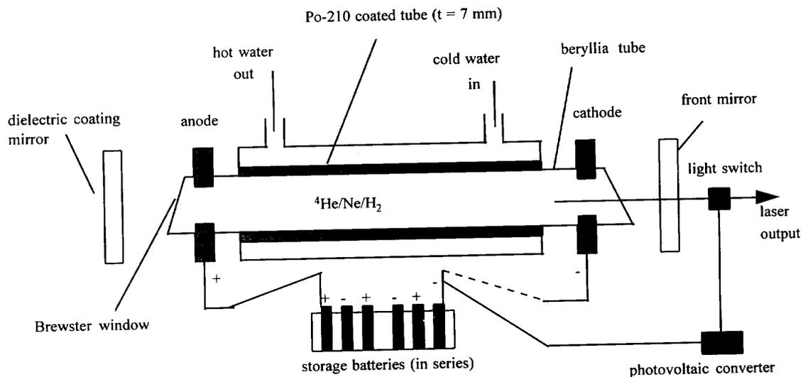
Figure 2. The main components of the radioisotope laser generator.
