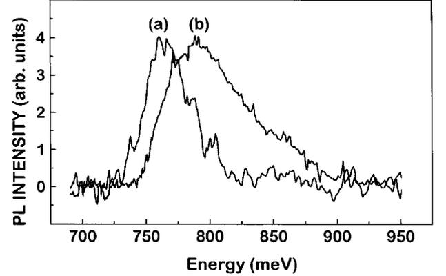
Figure 1. Room-temperature PL spectra of the InP-InGaAs AQW (nominal 100 Å wide) under low-excitation intensity (a) and high-excitation intensity (b).
