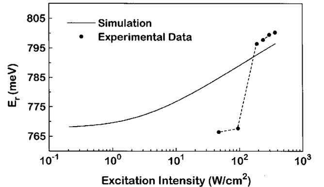
Figure 2. Photoluminescence recombination energy versus excitation intensity. The points are experimental results and the full line represents a simulation according to eqs. (1) and (2).
